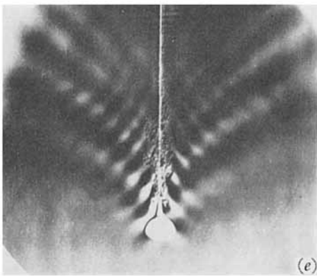
FIGURE 5. Experimental and theoretical wave patterns when \omega_0 = 1.14 rad/s. The scale marks represent a length of 5 cm. (a) and (b) V = 0.30 cm/s, N = 1.06 . (c) and (d) V = 0.55 cm/s, N = 1.37 . (e) and (f) V = 0.57 cm/s, N = 1.71 .
